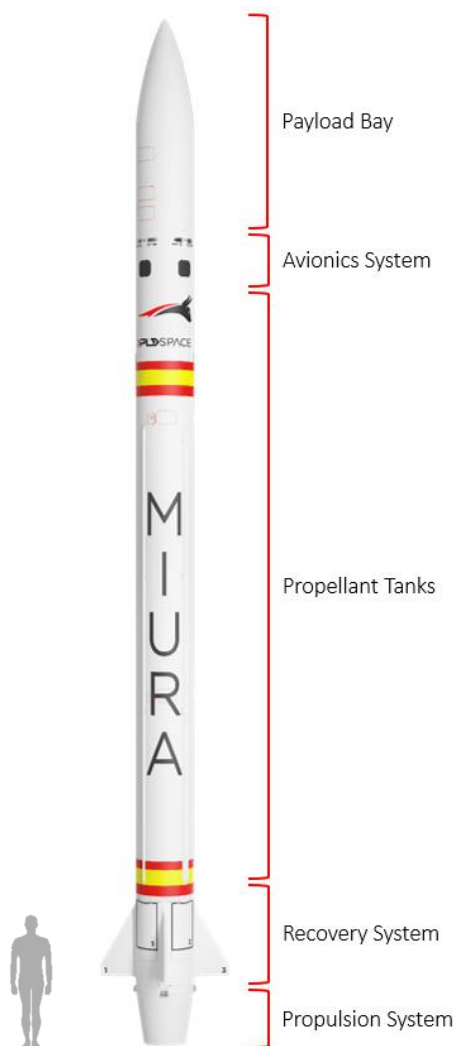
Figure 2-1 MIURA 1 Rocket and Subsystems
