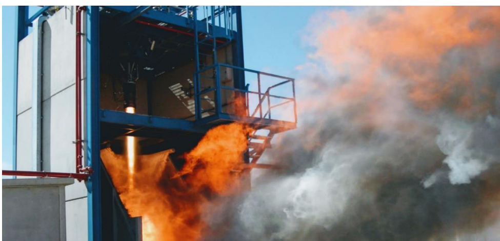
Figure 3-7 TEPREL Engine test at PLD Space’s Propulsion Test Facilities in Teruel
