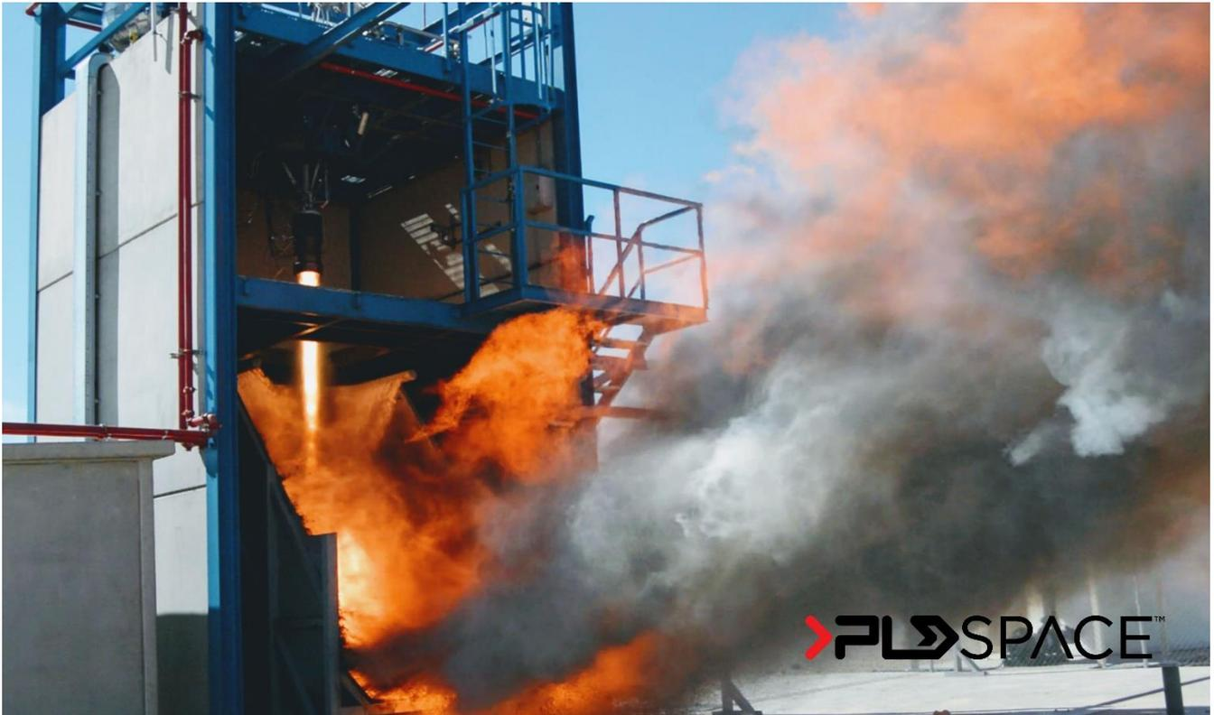
*Picture 1. Test Bench T1 during a hot test*
